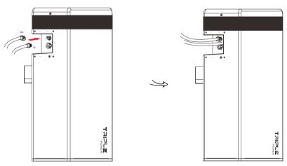
2. Keep the inverter off. Connect the other end of power cables (+,-) to the BAT (+,-) port on the inverter.
