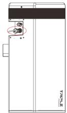
2. Insert the other end of the CAN communication cable to the CAN connector (II) on the first battey which is marked in red.
